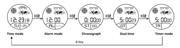
At any state ,press A or E key EL backlight for 2s.
